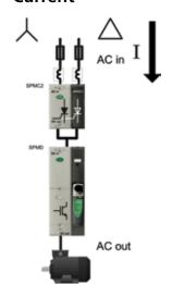
Multi-pulse rectifiers can be configured (12, 18 and 24 etc.), to minimise input harmonics and help to meet local supply authority regulations.
